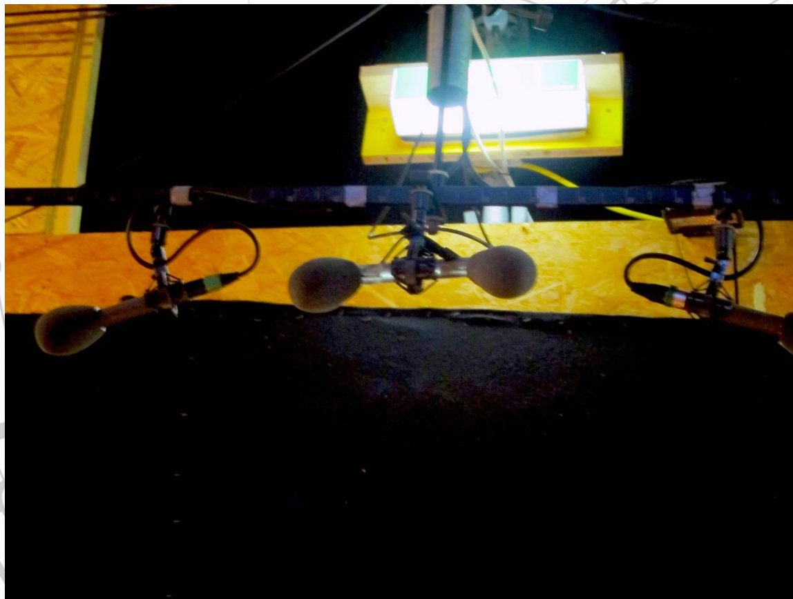
Extended OCT Main Orchestra Microphone with ORTF instead of center cardioid
