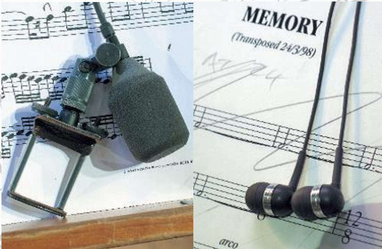
Schoeps String “Pick-Up” system/ IEM for orchestra
